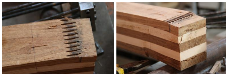
Fig. 3 - Local compression failure in beam ends ( L_{1-3-1} )
