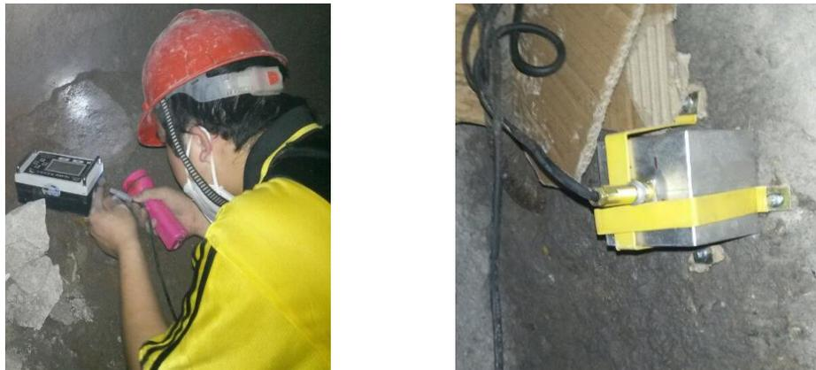
(a) Vibration meter host (b) Three-way vibration sensor
