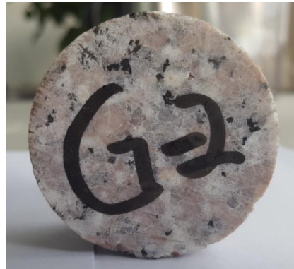
Fig.1 - Rock simple for Brazilian test
