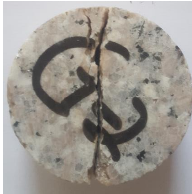
Fig.3 - Fracture pattern of BTS test
