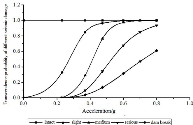
Fig. 7 - Seismic vulnerability curves of the Koyrna dam considering strain rate
