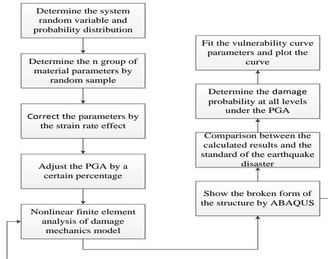
Fig. 5 - Procedure of seismic vulnerability analysis
