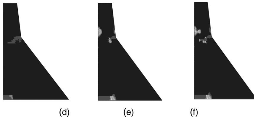
Fig. 2 - Failure modes of the Koyna dam
