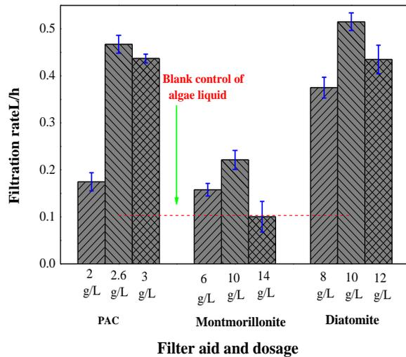
Fig.4 - Effect of Different Dipping Agents on Algae Water Filtration Rate
