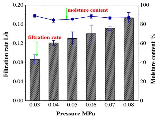
Fig.1 - Relationship between filtration rate and pressure in algae
