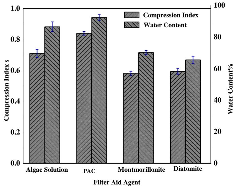
Fig. 11 - Effects of Different Aid Filter on Cyanobacteria Compression Index and Dehydration Efficiency
