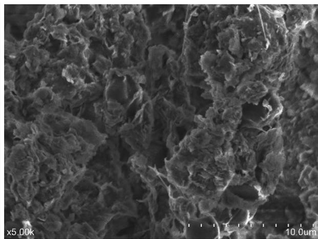
*Fig.8 - SEM images of Algae + Montmorillonite*
