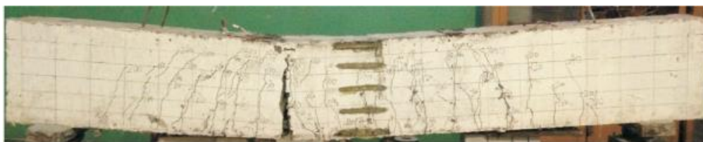
(a) B2~B6 BFRP rupture
