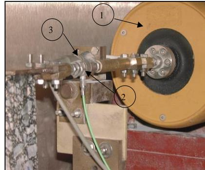
Fig. 2a - Specimen biasing device
