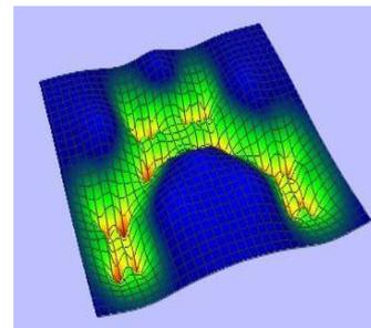
Fig. 3c - 3D graphical Visualization of deformations generated by a B747 aircraft (CESAR-LCPC) [29]
