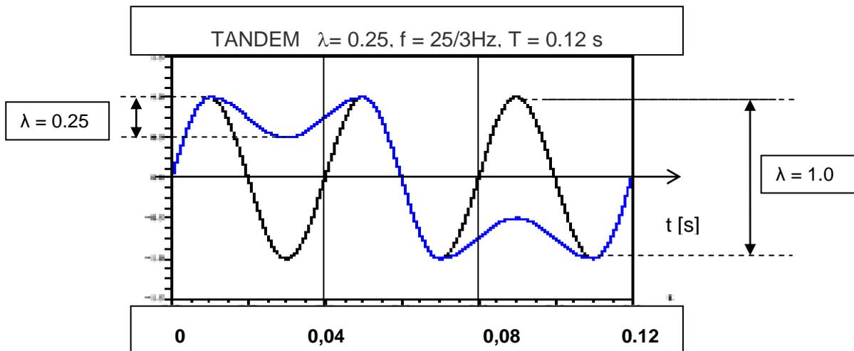
Fig. 1b - Illustration of Tandem\_0,25 signal
