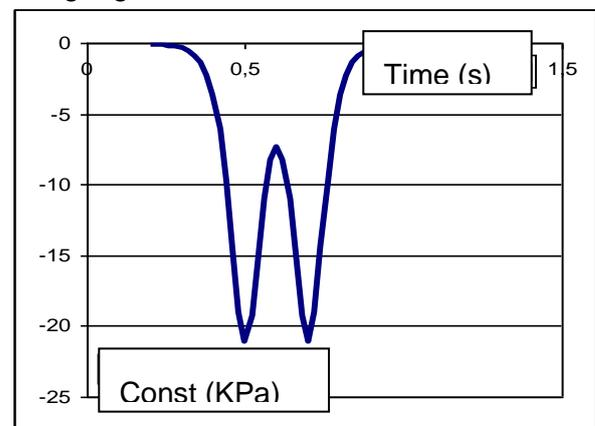
Fig.4b - Simulation of constraints evolution, according to Boussinesq
