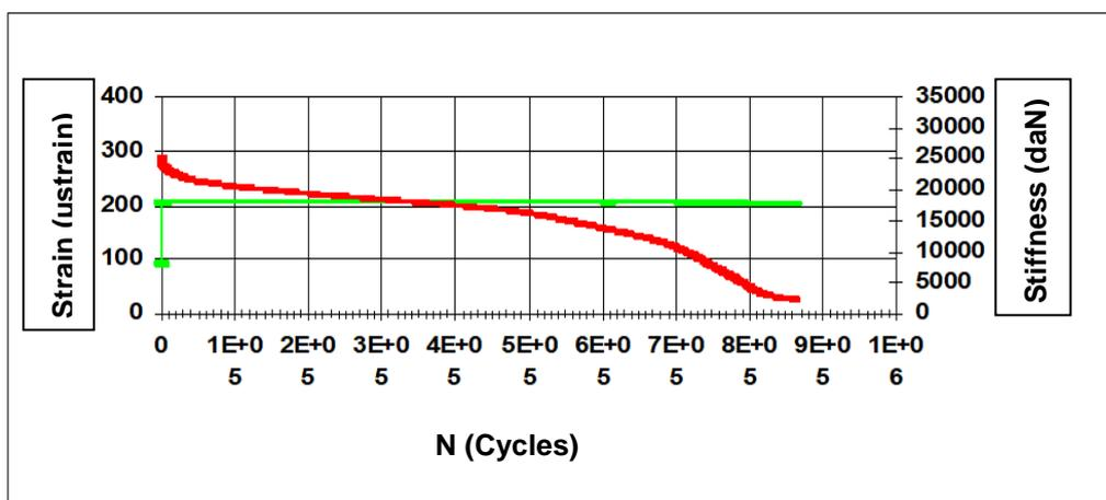
Fig. 6.a - Strain and fatigue curves of SINE Signal
