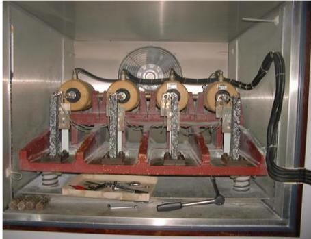
Fig. 2a - Machine test of fatigue
