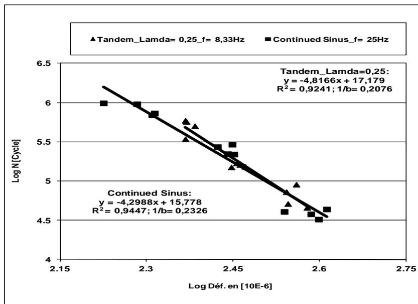
Fig. 7 - Fatigue laws for tandem\_0.25 and sine (tandem\_1.0)
