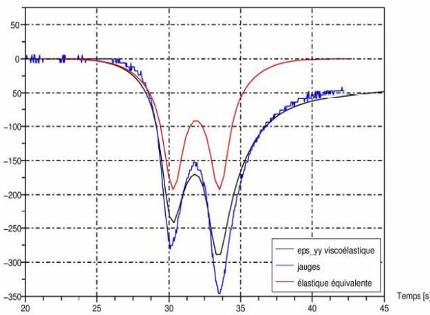
Fig. 4a- Elastic and viscoelastic simulations (Viscoroute) and transversal strain measurements at the bottom of bituminous layers [30]
