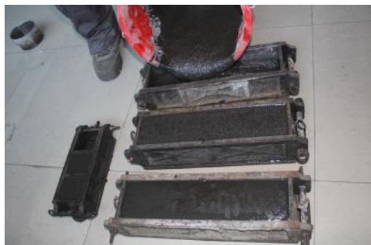
Fig. 2 - Casting drawing of specimens
