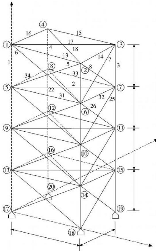
Fig.4 – structure diagram of the 72-bar spatial truss
