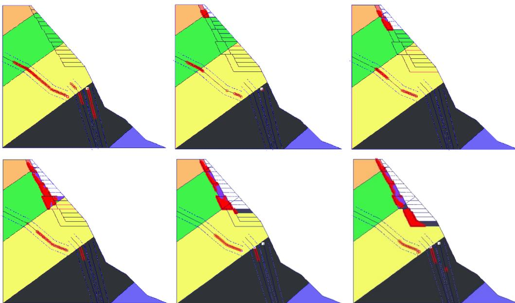
Fig.7 - The plastic points distribution of rock mass with considering unloading
