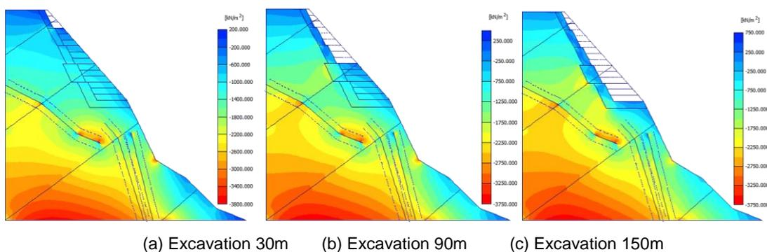
Fig. 5 - The average effective stress of rock mass with considering unloading
