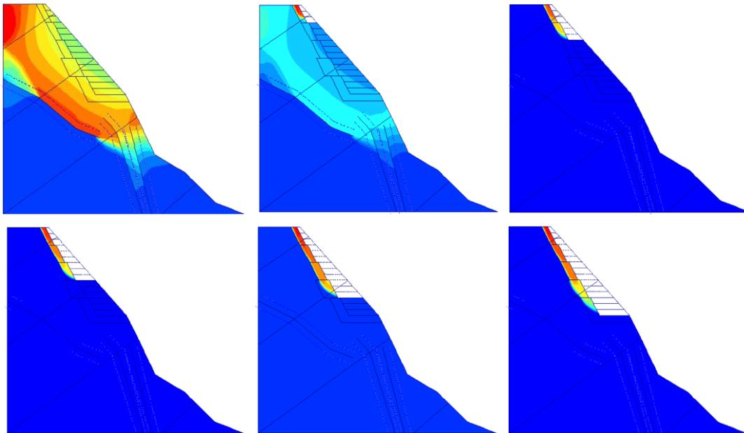
*Fig.9 - The slip surface of slope with considering unloading*
