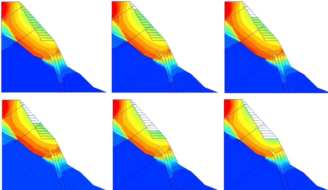
*Fig.8 - The slip surface of slope without considering unloading*
