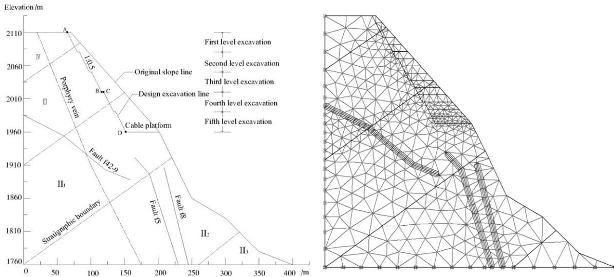
Fig.2 - Sketch diagram of slope excavation for cable crane platform of Jinping I Hydropower Station Fig.3 - Finite element mesh model and boundary of the slope
