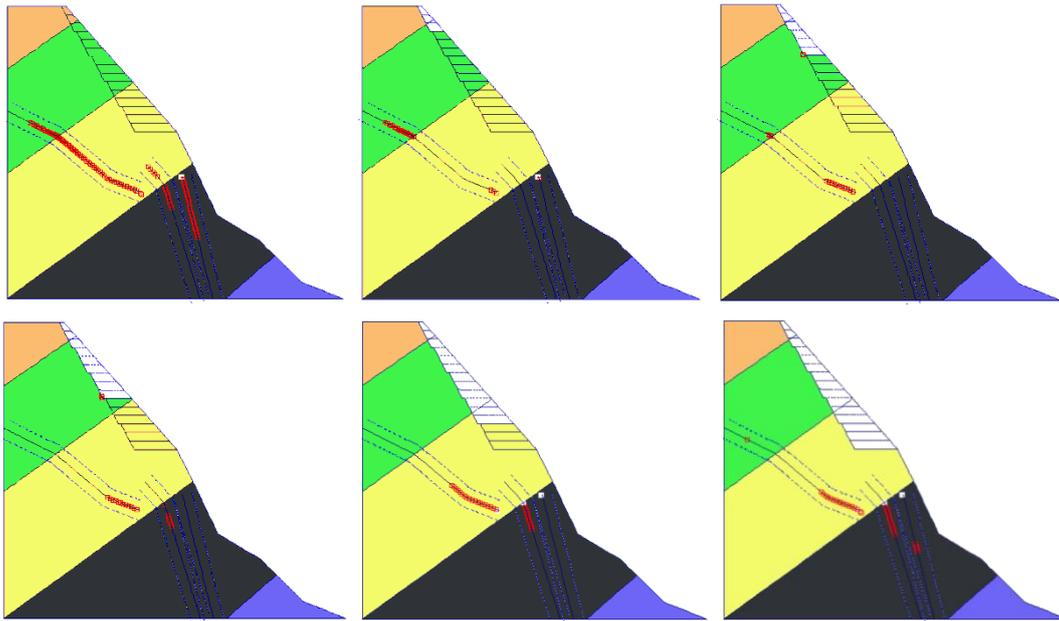
Fig. 6 - The plastic points distribution of rock mass without considering unloading
