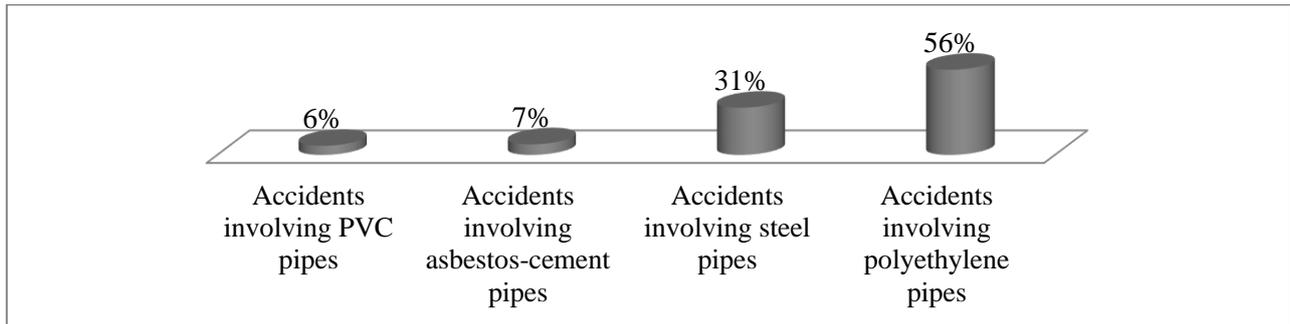
Fig. 3 – Various types of pipes involved in accidents in the water supply network
