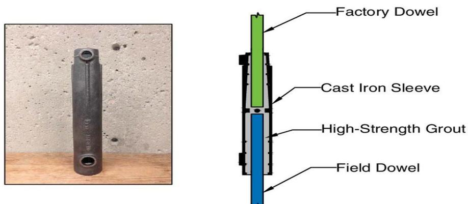
Fig.1- Elements of the GSS connector
