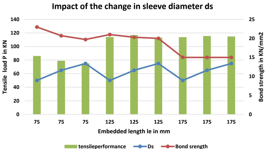
Fig. 5 - Impact of sleeve diameter
