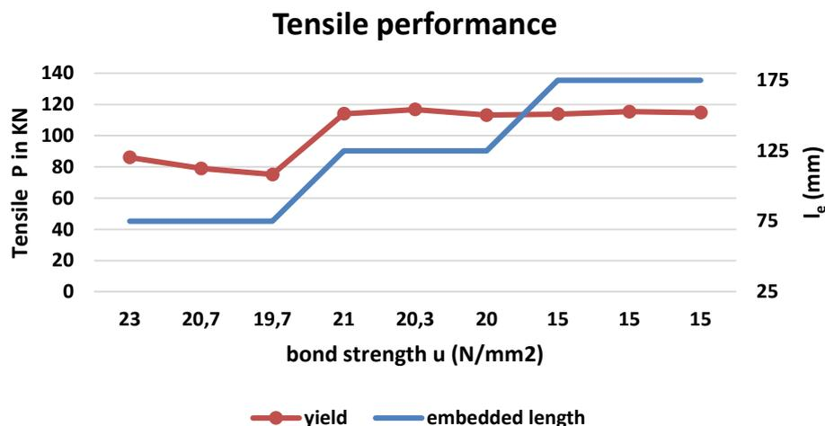
Fig. 3- Tensile performance for different embedded lengths
