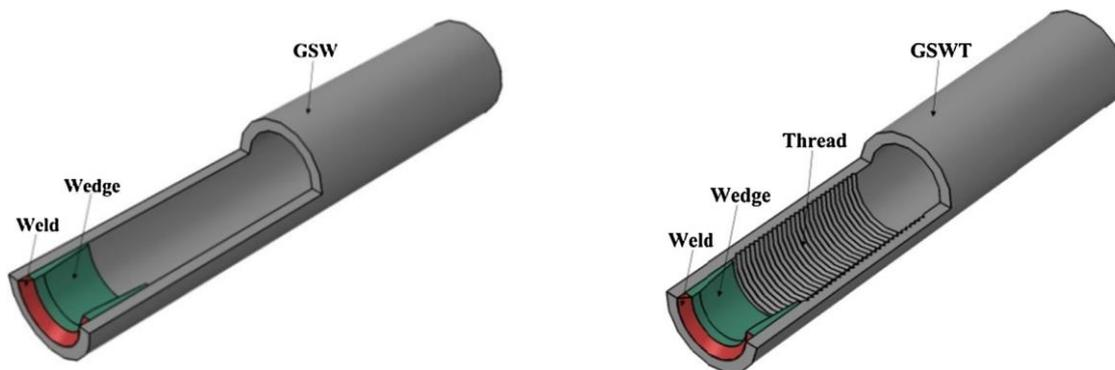
*Fig.6- Sleeve cylinder with wedge and with wedge and threads*
