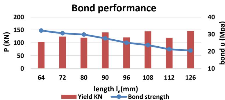
Fig. 2- Behaviour of bond strength under increasing embedded length
