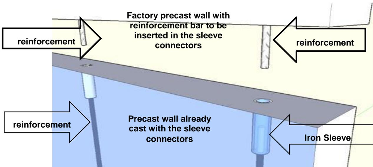
*Fig.2 - Erection of Precast members using grouted sleeve connector*
