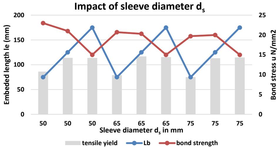
Fig.4- The impact of the diameter of the sleeve cylinder
